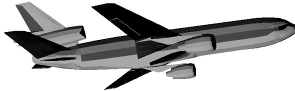
Figure 4: A CAD model as polygon soup
